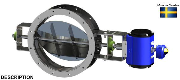
**Serie 200** is a very robust construction with a solid shaft penetrating the damper body. The two flanged bearings are mounted on brackets outside of the damper, preventing gas from entering the bearings.
