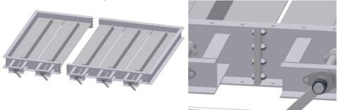
4. Use the bolts M 20 from the wooden box and bolt the 2 houses together. Use 160 Nm
