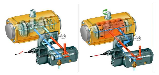
When no current is put through the solenoid, the springs inside the actuator force the air out to atmosphere and the actuator to its fail position.
